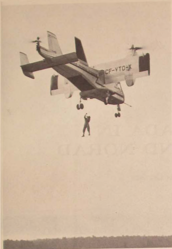
The CL-84 Dynavert, a VTOL craft developed jointly by Canadair and the Canadian Department of Defence, can rescue one to three men at a time from ground or water.
