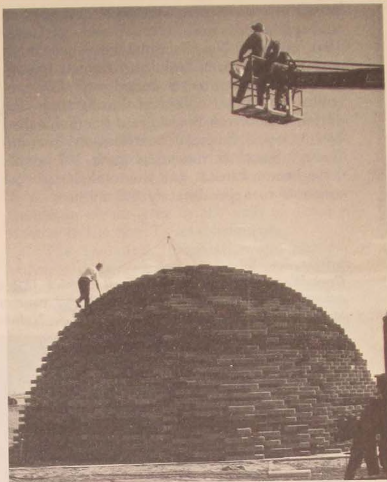
A 500-ton mound of TNT was detonated at DRB's prairie research station in 1964, with U.S. scientists and officers participating. The experiment yielded information on shock and blast effects of such explosions.
